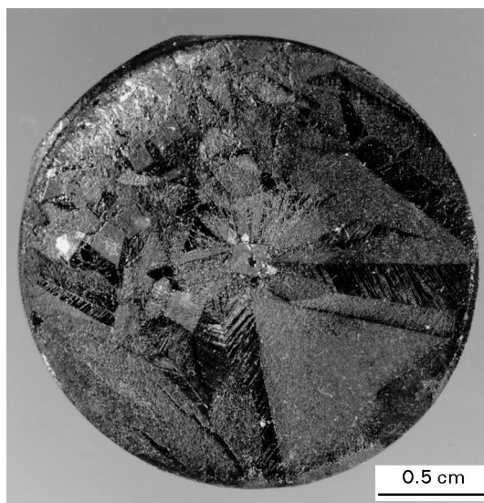
Figure 1 Photograph showing the melt-processed Sm-123 sample fabricated using a \text{SrTiO}_3 seed.
